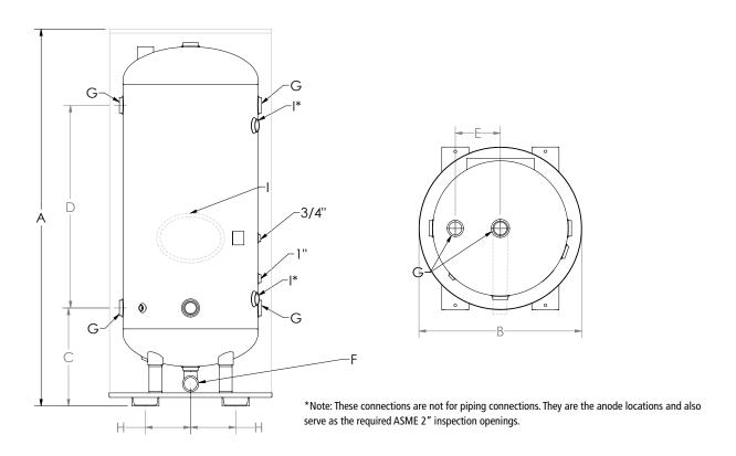
**NOTE:** Inspection openings i.e., 4" x 6" handholes and 12" X 16" manholes, are optional on diameters 36" and below and are to be included with tanks only when specified.
